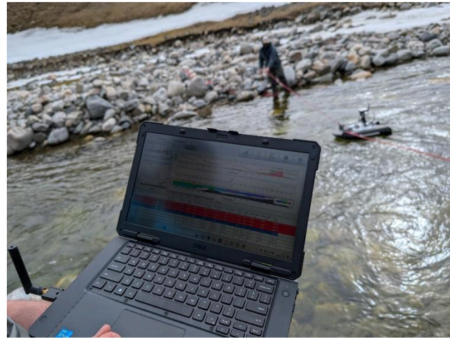
Figure 12. Logan helps to guide the Acoustic Doppler Current Profiler (ADCP) across the stream while Eric reviews the real-time stream profile data. (CC BY-NC-SA 4.0: W. Ray)
