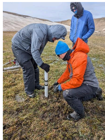
Figure 9. Left photo: Eric and Logan drill into the active layer to install the groundwater well. Right photo: Installing the groundwater well. (CC BY-NC-SA 4.0: W. Ray)
